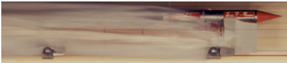
Figure 1.3 SRR Sled at 4,865 fps in Air (Mach 4.3)
